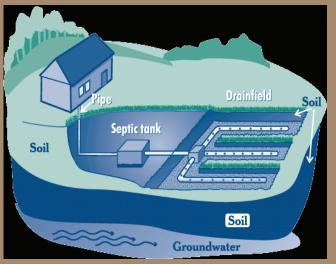
The most common sewage treatment system contains a septic tank and leach lines, or trench, as shown in the picture. All wastewater stays underground and is treated by filtering through
